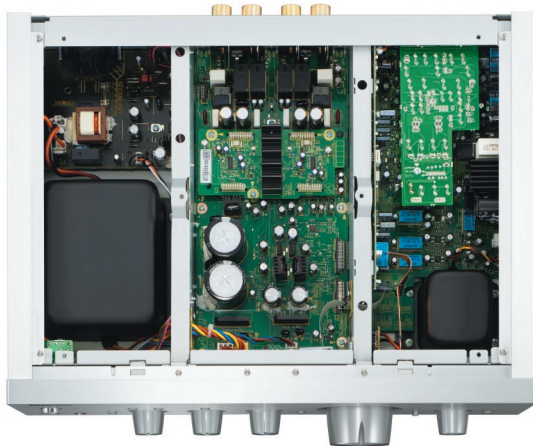
Three Chamber Construction
