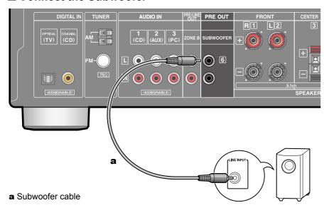
Connect a supplied powered subwoofer with this unit using a subwoofer cable. Up to two powered subwoofers can be connected (Purchase a second powered subwoofer separately). The same signal is output from each SUBWOOFER PRE OUT jack.
