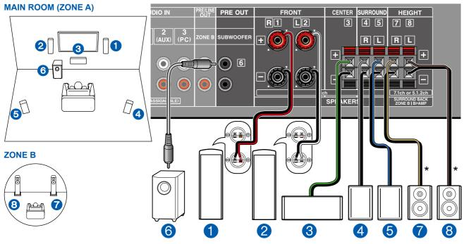
MAIN ROOM (ZONE A): For details of the speaker layout, refer to "Speaker Installation" ( $\rightarrow$ p23).
