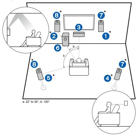
This is a 5.1.2 Channel System that uses the supplied center speaker and powered subwoofer in combination with a separately available speaker system. Dolby enabled speakers, which are types of height speaker, are special speakers designed to face the ceiling so that sound is heard after bouncing off the ceiling so that sound appears to be coming from overhead.
