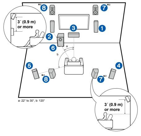
This is a 5.1.2 Channel System that combines the supplied speaker system with separately available front high speakers or rear high speakers.
