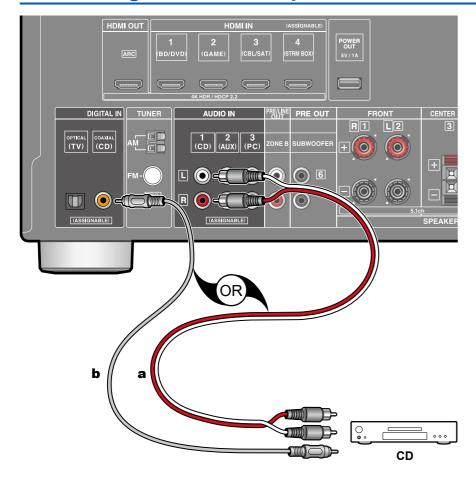
This is a connection example of an audio component. Connect a CD player using a digital coaxial cable or analog audio cable.
