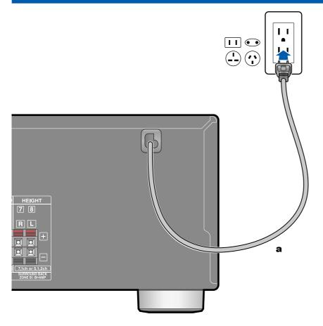
Connect the power cord after all the connections are completed.
