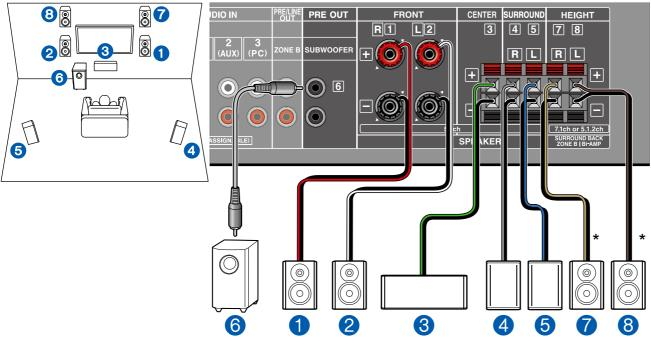
This is an example of a 5.1 Channel System combined with separately available height speakers. You can select one combination from the following 3 types according to the type of height speakers to be used and the usage environment, then make the connections.
