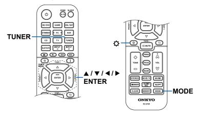
When FM broadcasts reception is poor: Perform the procedure for "Tuning Manually" ( $\rightarrow$ p52). Note that if you tune manually, the reception for FM broadcasts will be monaural rather than stereo, irrespective of the sensitivity of the reception.
