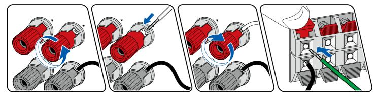
Make correct connection between the unit's jacks and speaker's jacks (+ side to + side, and - side to - side) for each channel. If the connection is wrong, a bass sound will not be reproduced properly due to reverse phase. The wires exposed from the tip of the speaker cable do not stick out of the speaker terminal when connecting. If the exposed wires touch the rear panel, or the + side and - side wires touch each other, a malfunction may occur.
