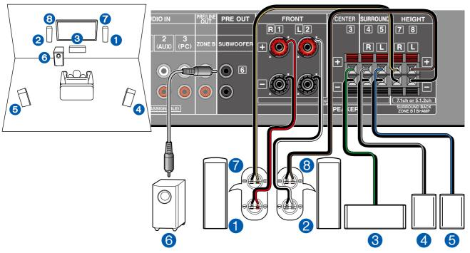
$\square$ Example installation when the entire supplied speaker system is connected( $\rightarrow$ **p26**)
