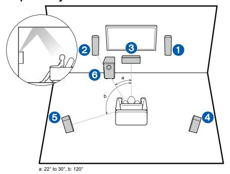
This is a 5.1.2 channel system where the entire supplied speaker system is connected.
