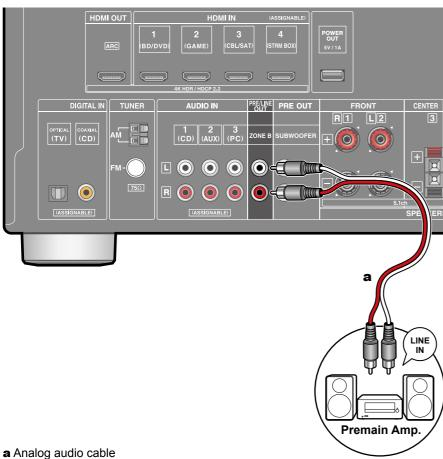
While performing playback in the main room (ZONE A), you can enjoy 2-ch audio of the same source in the separate room (ZONE B) at the same time. Use an analog cable to connect the ZONE B PRE/LINE OUT jack of this unit and the LINE IN jack of the pre-main amplifier or power amplifier in the separate room.
