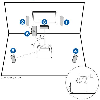
Front speakers output the front stereo sound, and a center speaker outputs the sound of the center of the screen, such as dialogs and vocals. Surround speakers create the back sound field. Powered subwoofer reproduces the bass sound, and creates the rich sound field.
