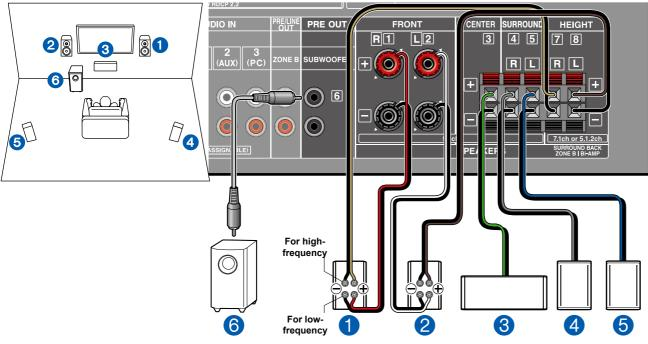
You can configure a 5.1 Channel System ( $\rightarrow$ p23) by connecting front speakers that support Bi-Amping connection. The Bi-Amping connection can improve the quality of the low and high pitched ranges. Be sure to remove the jumper bar connecting between the woofer jacks and tweeter jacks of the Bi-Amping supported speakers. Refer to the instruction manual of your speakers as well.
