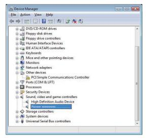
If the [Pioneer xxxxxx] does not appear, confirm that the USB-B port has been selected as input source. Then try reconnecting the cable or turning the power off and then on again; when this is done, the [Pioneer xxxxxx] should be recognized.
