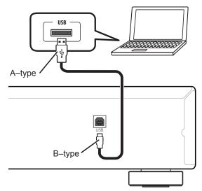
\* The port used to connect the computer with the product's main unit is called the "USB-B port" in this manual. The actual name and location of the port will differ from product to product.
